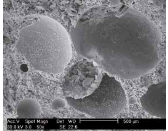
Picture 1 Macropores in dehumidifying mortar from the Mape-Antique range.
