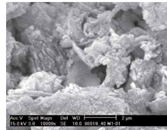
Picture 3 Micrograph of ancient mortar. Notice how the amorphous mass is completely carbonated.
