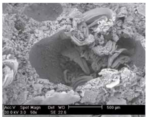
Picture 2 Crystallisation of salts in the macropores of dehumidifying mortar from the Mape-Antique range.
